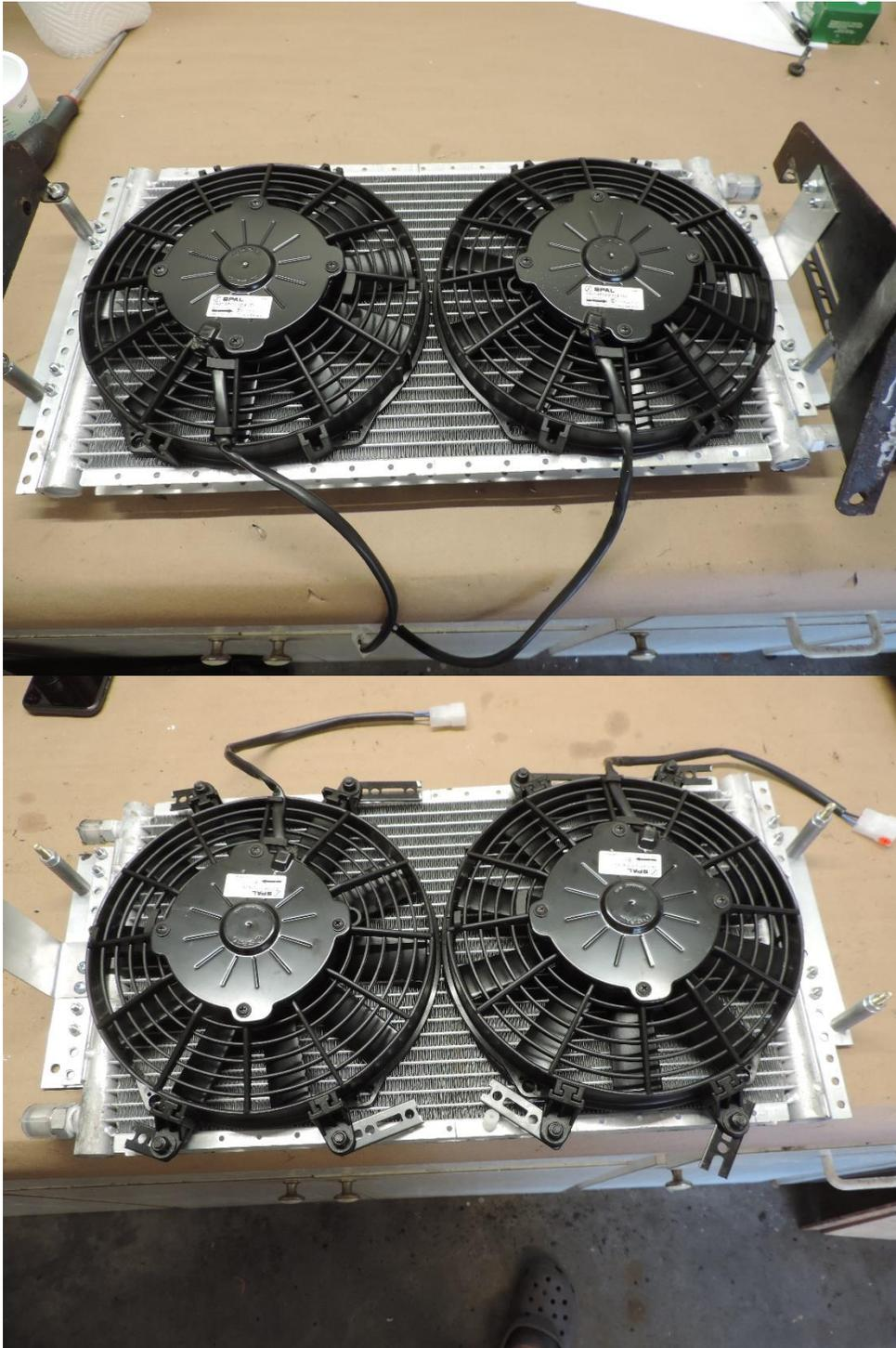
The fans are SPAL fans VA07-AP12/C-31S or 30100381, 9" diameter.
